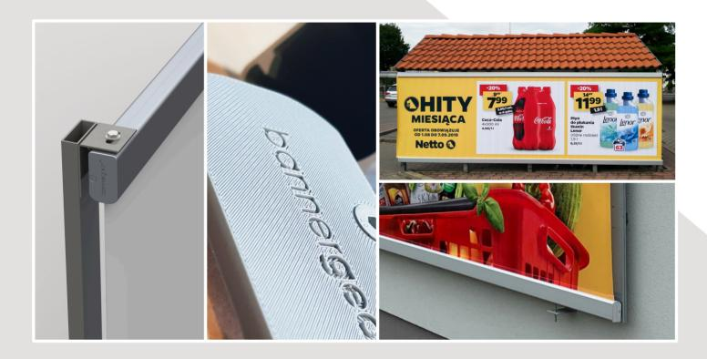
Slide system model of bannergear™ system is made from two parallel profiles between which the advertising banner is placed. The system allows you to optimally tighten the printout and display your advertisement without the use of tools. Banner is printed on vinyl with kedra endings, thanks to this idea, the banner has a uniform surface and fits perfectly with the aluminum guides. Profiles made of anodized aluminum make the structure light and resistant even to the worst weather conditions.
