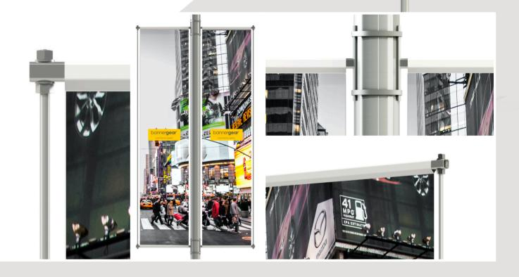
Bannergear™ system Wing Frame model is designated for mounting on lanterns, poles near restaurants, gas stations or similar. Intended for displaying two-sided banners. Carrier structure is made from steel profiles ended with adjustable steel clamp ring. Banner is stabilized and regulated by threaded steel rod complete with counter screws.
